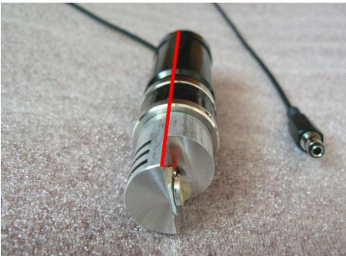
Now you have to align the flat side of the LED lamp to the positioning strip at the rear of the black holder, like in the image.
