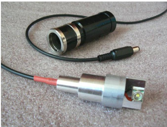
The LED lamp has a cord with a plug, insert the plug from the front into the holder, so it will come out at the other end
