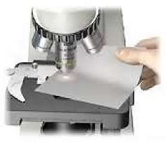
Check the centering with a low mag objective, see if the spread is even. (assumed that your light system (substage condensor) is centered)
