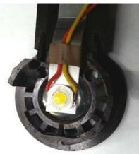
The LED, The yellow dome can now be positioned above the center of the mirror, this is a good starting position for later adjustment.
