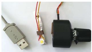
The microscope was modern for its time, with the halogen lamp, but we find more and more problems in supplies and lampbases, parts are getting harder to find. So we developed this LED light set, the LED gives (much) more light at a better color, and is just like the halogen adjustable in intensity.
