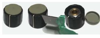
You can take the intensity knob from the scope's base, by lifting the cover, and loosen the nut (with a flat plier or pipe wrench) the nut does not have to be removed, just loosened, you can lift the knob from the axel of the regulator.
