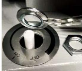
Turn the white axel of the dimmer in the off position, (click, CCW) now you can put the knob on the axel, whit the arrowpoint at the "off"sign. Lift the knob 1 mm while fixing the small srew in the knob. ( if the knob is scratching the surface or the nut, when turned, please lift it another mm.)
