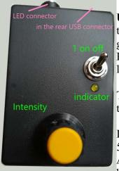
Using the dimmer, When connected to the COB and (powered) USB, the dimmer can be switched on with the switch (1) the yellow indicator goes on.
