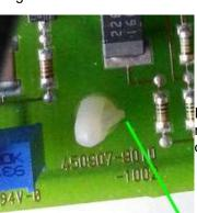
If all wires are from the old to the new board, take the plier and squeeze the nose of the plastic clip, while lifting the board, same at the other end...... the old board is free, now you can clip on the new borad on the plastic clips.
