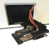
The lamp has a white wing which is between two contact layers, slide that out, to the front of the holder.
