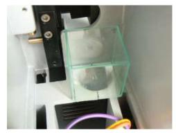
Take the regulator, witch has now three cables, lead the regulator with these cables in a slow curve into the green cube. By means of a magnet, the regulator will stick at the bottom. (if needed you can use the tie-rap to hold the cables, loose fit)
