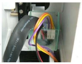
Swing the back plate of the microscope back to its orriginal position, mind that the cables don't intefere with the mechanics, and put in the 4 srews and screw tight
