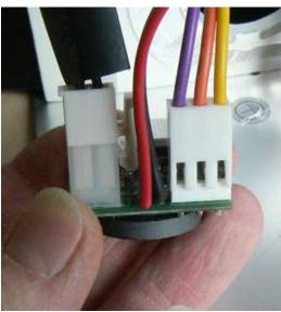
Next to the metal of the regulator you find two new sockets where you can fit both cables that you just have taken out of the microscope board
