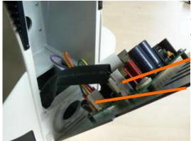
Now you can carefully open the rear of the microscope which is still connected with a few cables to the electronics board.
