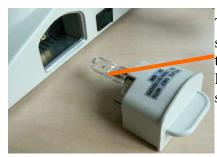
Take out the lampholder from the side of the microscope base, take out the halogen bulb and put in the LED Lamp at the vacant position. (sticker side up) fit the lampholder again.
